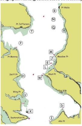
Bearings are magnetic. Distances are nautical miles (NM). Bearings, distances, and positions are approximate. Each temporary mark is shown with its label in a circle. Each permanent mark is near its label in a square box.
